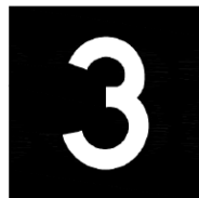
Runway Distance Remaining Sign
