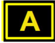
Taxiway Location Sign
