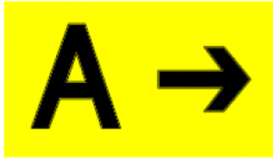
Direction/Runway Exit Sign
