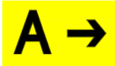
Direction/Runway Exit Sign
